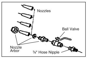
**Figure 3.** Sand blaster handle and nozzle assembly.
